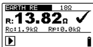
Figure 5.32: Example of earth resistance measurement result
