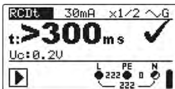
Figure 5.19: Example of trip-out time measurement results
