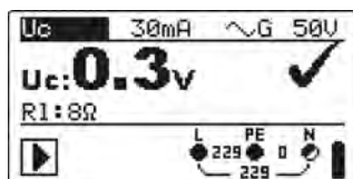
Figure 5.18: Example of contact voltage measurement results
