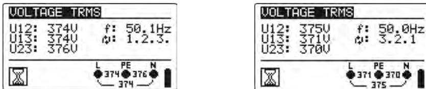
Figure 5.4: Examples of voltage measurement in three-phase system
