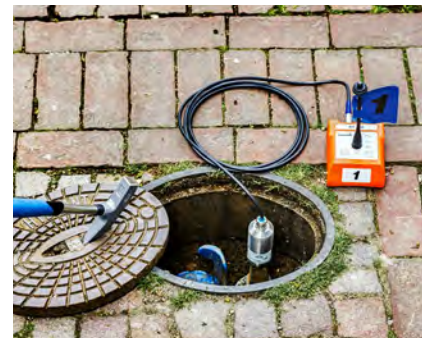
Performing correlation with the RT 200 radio transmitter and the UM 200 universal microphone
