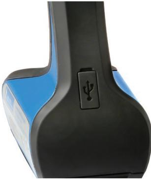
Fig. 11: Rear of the detector, with USB port
