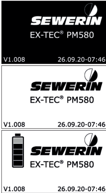
Fig. 9: Sequence of start images during switch-on process The logo can be customised using the GasCom software.
