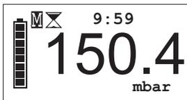
The measurement is started. The measured values and the remaining measurement time are indicated.
