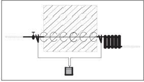
Fig. 3: Direct galvanic connection via conductor loop
