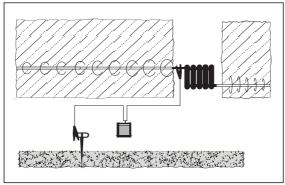
Fig. 4: Direct galvanic connection with earthing spike
