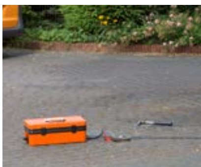
Acoustic location of main pipes
