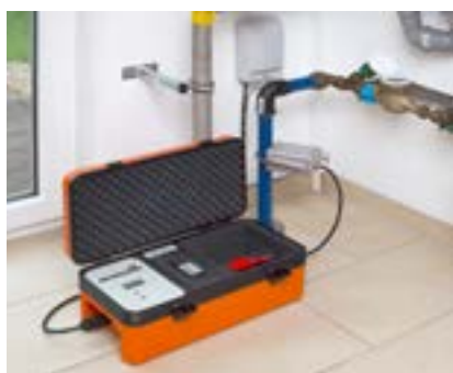
Locating metallic pipes and plastic pipes
