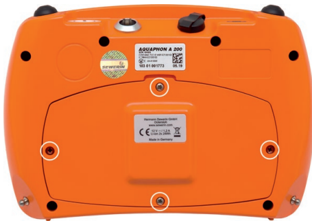
Fig. 32: Back of the A 200 receiver White circles: Screws of the battery compartment cover
