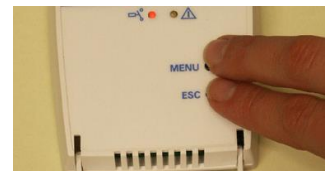
Figure 5 The ENTER command is done by pushing buttons MENU and ESC at the same time for about 14s.
