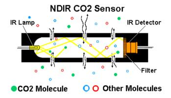
As shown in the figure, gas molecules diffuse into the sensing chamber. The IR light is directed through the sensing chamber towards the detector. The detector has a filter in front of it which eliminates all light except the 4.26  $\mu$ m wavelength that CO<sub>2</sub> molecules can absorb. Since other gas molecules do not absorb light at this wavelength, only the CO<sub>2</sub> molecules affect the amount of light reaching the detector.
