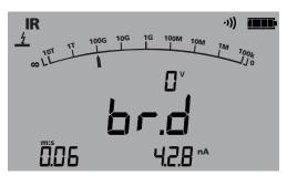
Burn mode disables the normal breakdown detection and test voltage continues after breakdown of the insulation. This enables the location of a failure to be detected but it is a destructive test.
