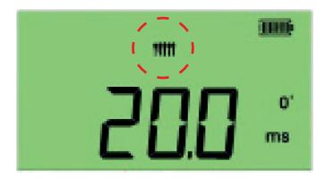
DC sensitive RCDs are tested as per standard RCDs. The RMS current used is  $\sqrt{2}$  x the rated operating current of the RCD.
