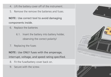
CAUTION : Do not over tighten the screws as this could damage the threat
