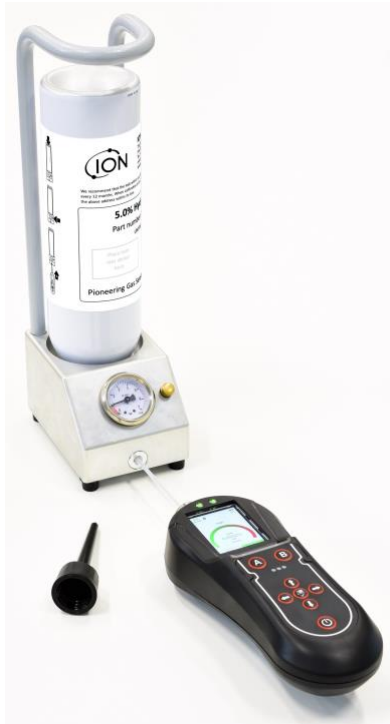
Figure 3: bump test / response check of a Panther leak detector
