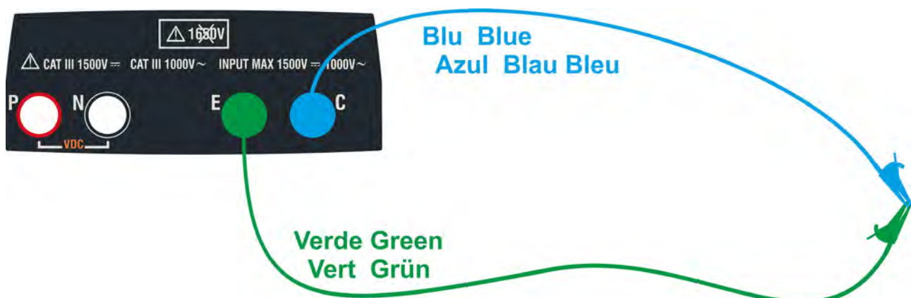
Fig. 4: Compensation of the measuring cables resistance
