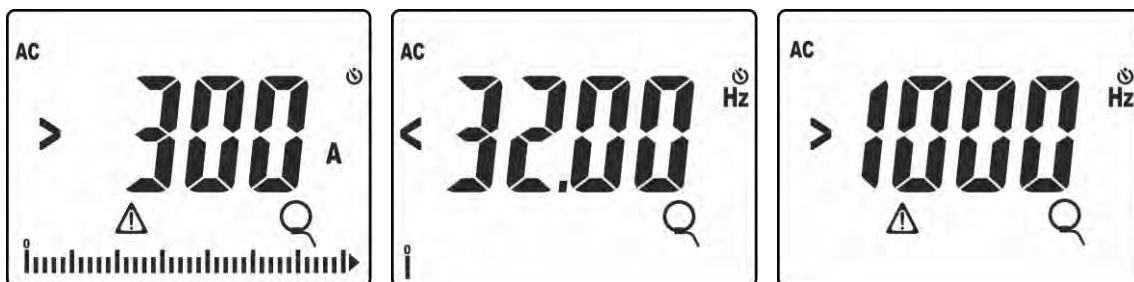
Fig. 39: Anomalous situations on current measurement with clamp transducers
