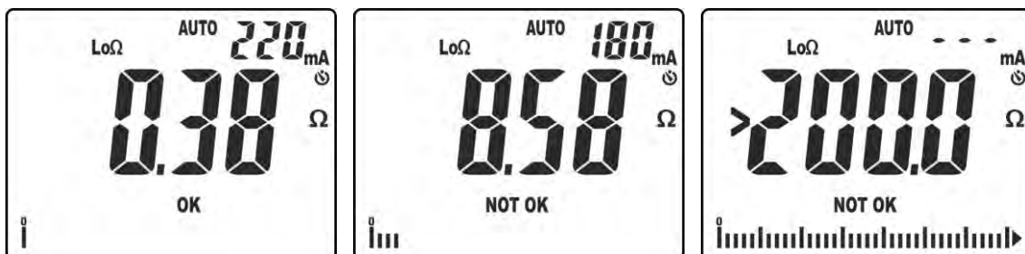
Fig. 28: Results of continuity test in AUTO mode
