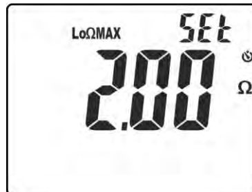
Fig. 26: Setting the limit threshold for continuity test
