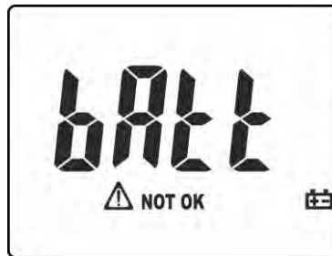
Fig. 43: Screen with low battery indication
