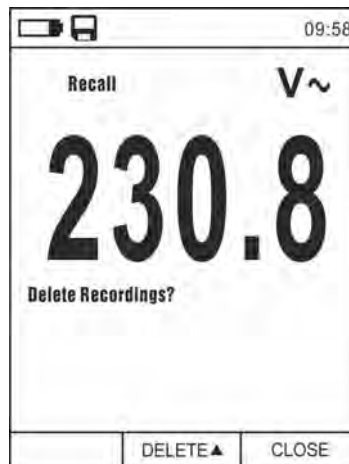
Fig. 36: Data logger function – Deleting recorded data
