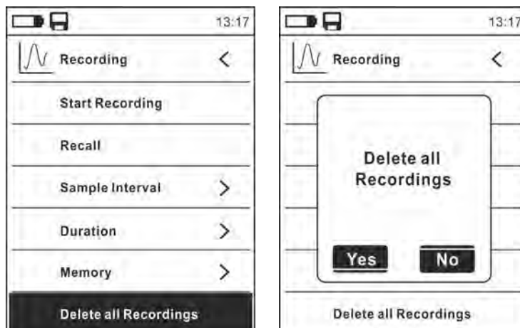
Fig. 38: Data logger function – Deleting all recordings
