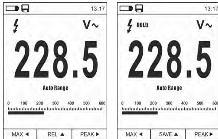
Fig. 7: Saving the value frozen on the display
