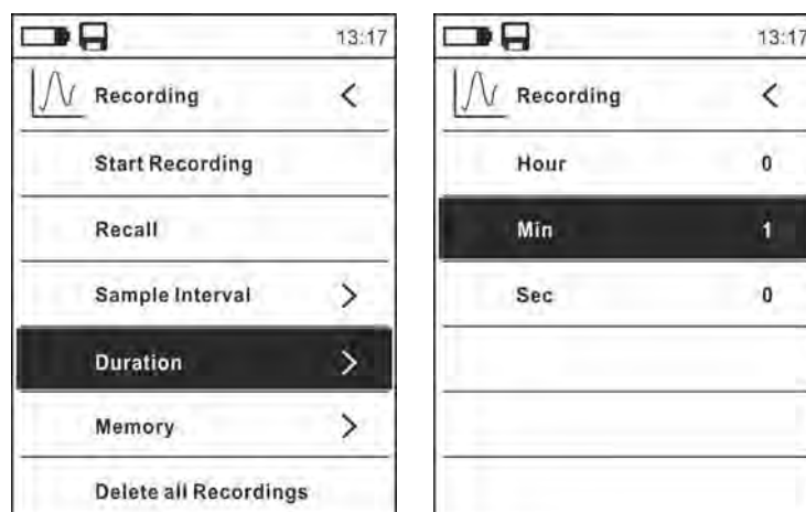
Fig. 32: Data logger function – Setting of recording duration
