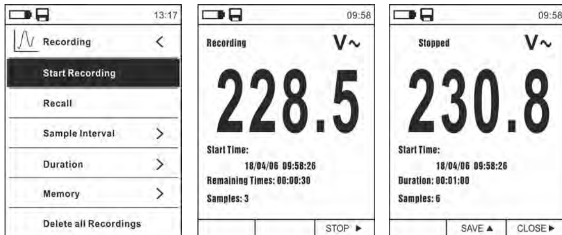
Fig. 33: Data logger function – Starting and stopping recording
