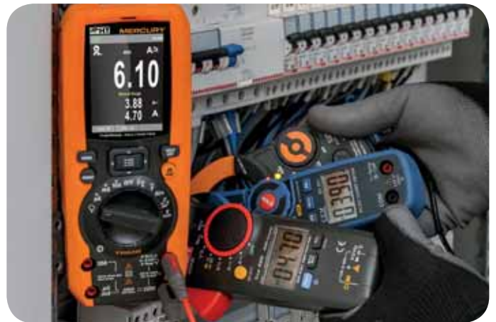
AC+DC current measurement comparison: 3.9A with RMS clamp, 4.7A with TRMS clamp, 6.1A with AC+DC TRMS clamp.
