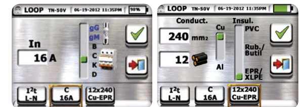
Setting of MCB/fuse type and rated current
