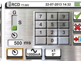
Setting of RCD delayed time
