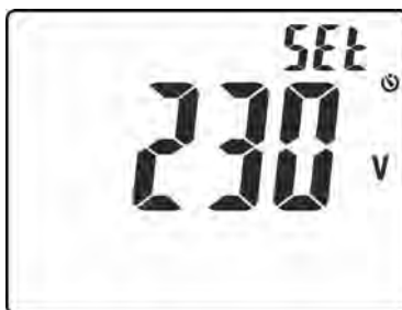
Fig. 6: Setting the rated voltage in Loop measurement
