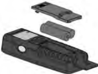
Fig. 14: Replacement of the internal battery
