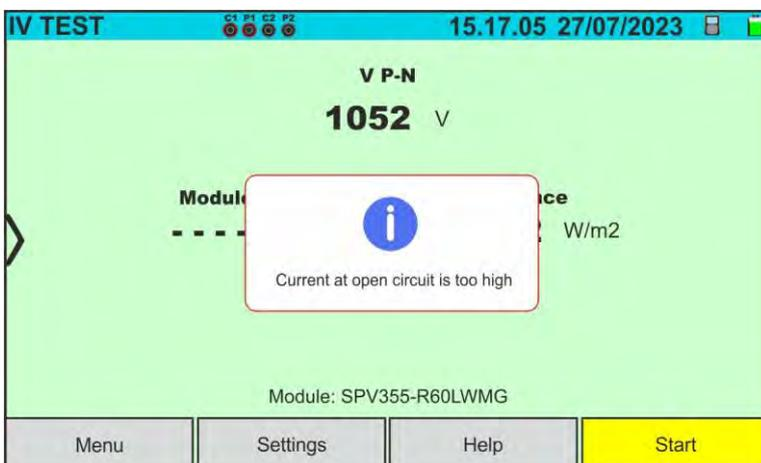
In the I-V curve measurement, if the current detected at the Voc point (no-load situation) is greater than 0.2A, the instrument does not perform the test and displays the message shown in the screen alongside. Check the circuit being measured and repeat the test.
