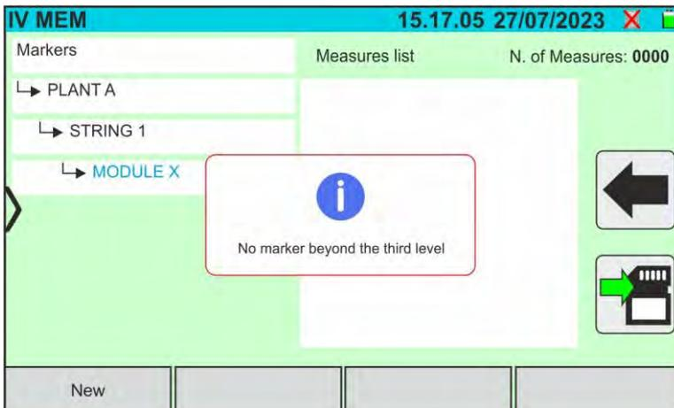
When the third-level marker is selected, touching the "**New**" key will display the screens shown in the figure and the instrument will not perform the operation. **It is not possible to define markers beyond the third level**
