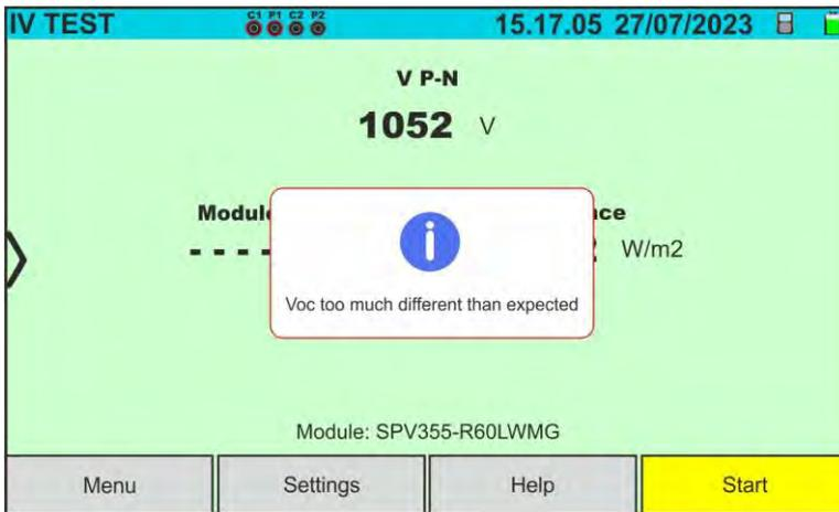
If, during the execution of an I-V or IVCK measurement, the open-circuit voltage ( $V_{oc}$ ) value is very different from that defined in the module database, the instrument does not perform the measurement and displays the message shown in the screen alongside. Check the values of the  $V_{oc}$ ,  $TC(V_{oc})$  parameter within the database and the number of modules set in the measurement
