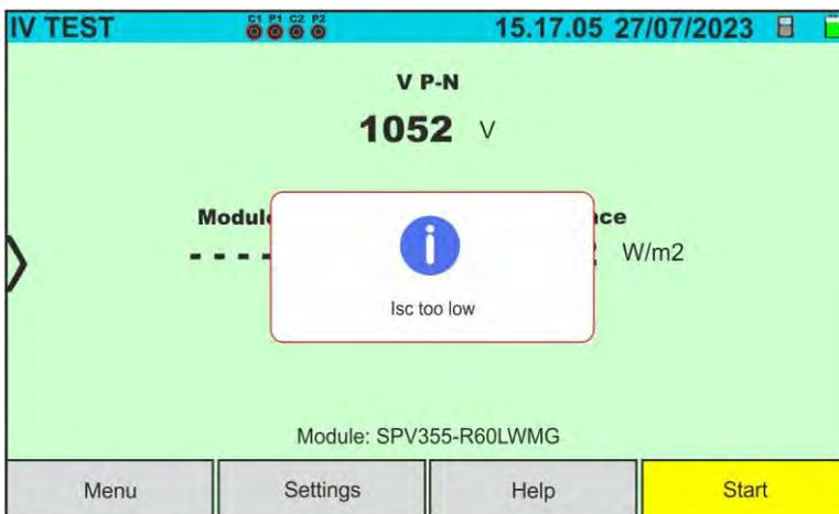
If the instrument detects a short-circuit current **Isc** below a **threshold limit**, it does not perform the test and displays the message shown in the screen alongside. Check the connections of the instrument, the functionality of the module/string, the module settings and the number of modules
