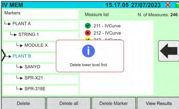
If a highlighted top-level marker containing some measurements is to be removed, the instrument will not proceed and will display the message shown in the figure. **Remove all lower-level markers first**
