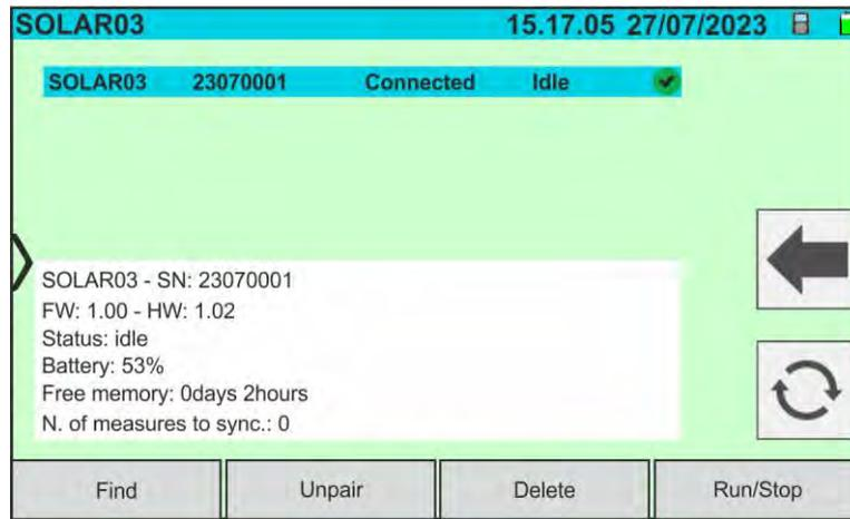
Fig. 18: Pairing a SOLAR03 remote unit - Step 4
