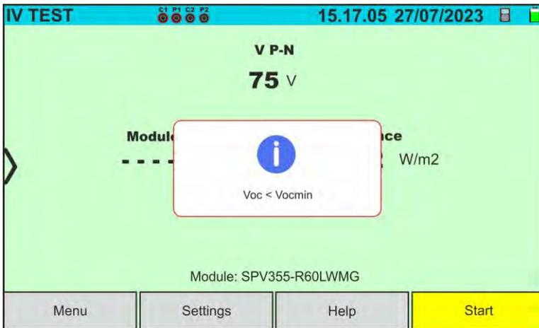
If the instrument detects, at the end of the test, a Voc too much different from the open-circuit voltage measured before starting the test, the message alongside is shown on the display. This condition could be due to the execution of tests on poor quality modules and/or too low short circuit current and/or measurements carried out with too low irradiance.
