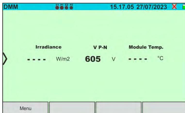
Fig. 14: DMM function measurement screen (SOLAR03 disconnected)
