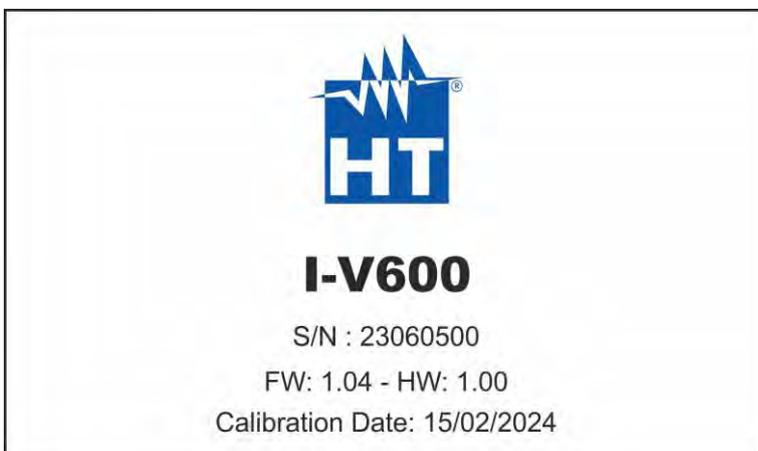
When switched on, the instrument briefly displays the initial screen before switching to the main menu. It shows:
