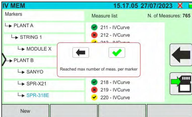
If, during saving, you try to associate a measurement with a marker in which the maximum number of possible measurements are present (**max 500**), the instrument shows the message shown in the figure on the side and does not carry out the operation. Download the measurements to the PC and delete them before saving again
