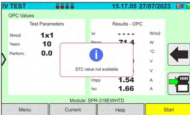
If, during the execution of an I-V or IVCK measurement, the instrument is unable to determine the @STC values, it displays the message shown in the screen alongside. Check that you have stable irradiation, in addition to the correct exceeding of the minimum threshold and that you have carried out the measurement in accordance with the indications of the M304 accessory (see § 6.4.2 – point 10). Repeat the measurements at other times of the day if necessary
