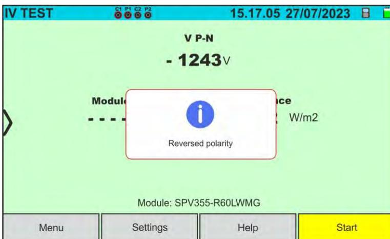
If the instrument detects a voltage  $< -0.5VDC$  at the P-N terminals of the string, it does not perform the test, emits a prolonged audible signal and displays the message shown in the screen alongside. Check the connections of the string poles
