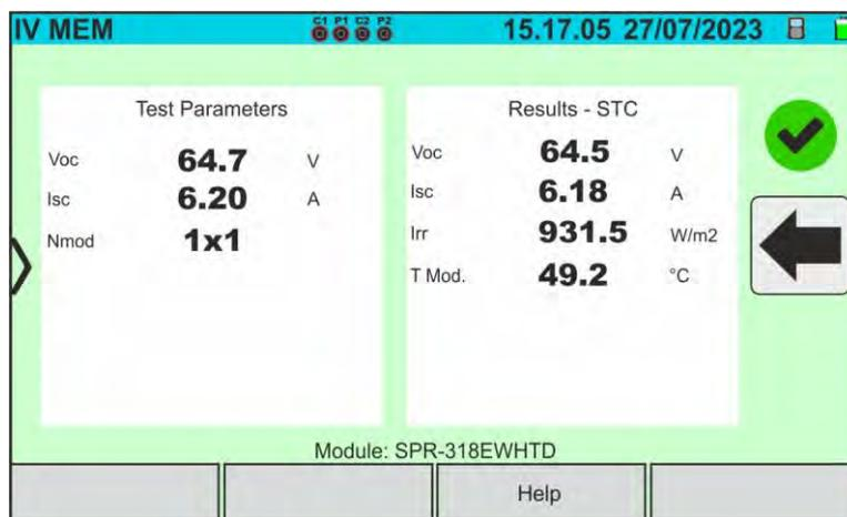
Fig. 78: Retrieving the IVCK test results @STC
