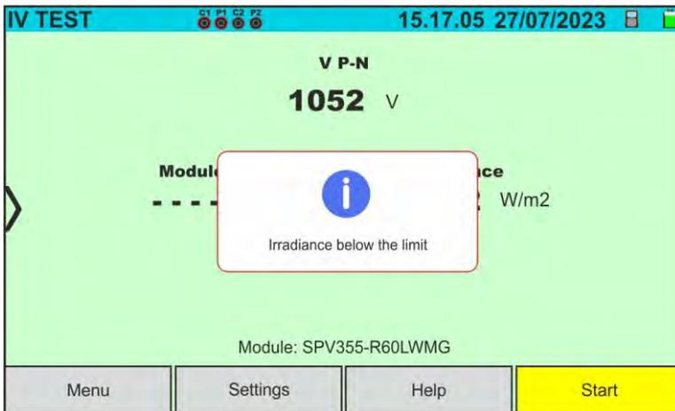
If, with the remote unit active and connected (even in recording mode), the instrument detects an irradiance value below the threshold (see § 5.2), it stops the test and returns to the main screen. Check the threshold value and carry out the tests at another time of the day with stable irradiation
