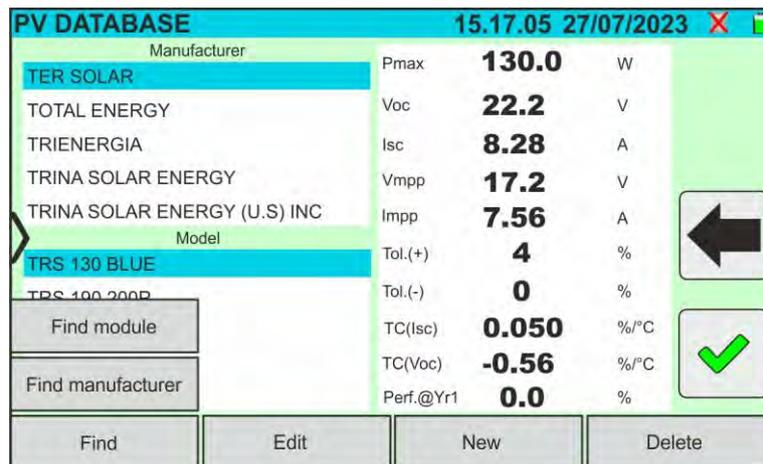
Fig. 29: Searching for a module in the database
