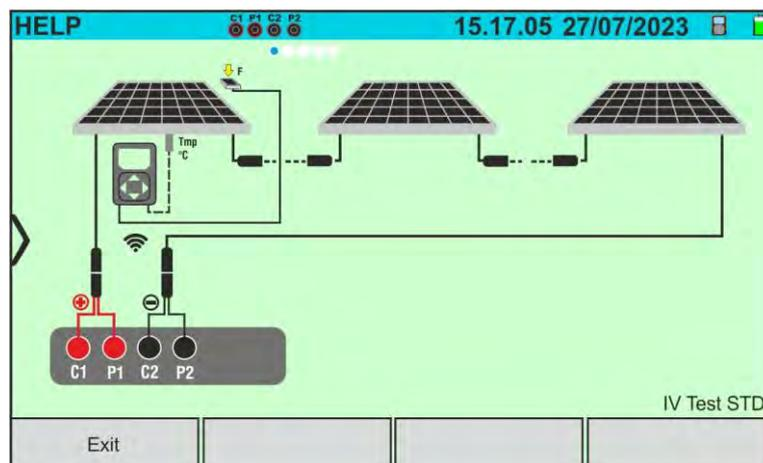
Fig. 9: Help screen for connecting to the instrument
