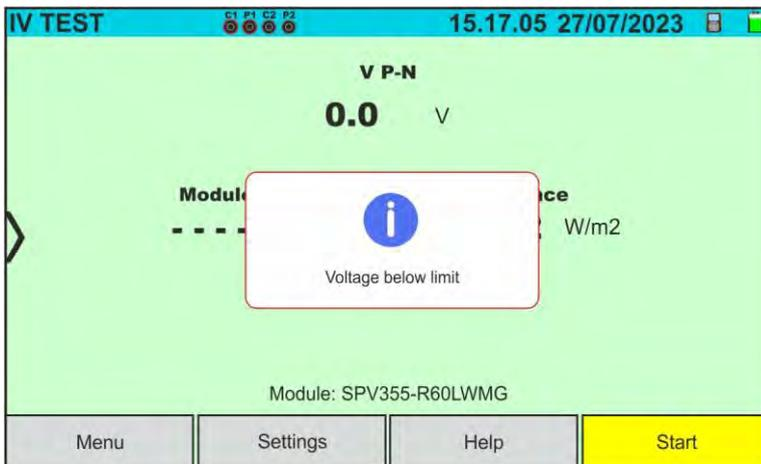
If the instrument detects a voltage of  $-0.5V \leq V_{PN} \leq 15VDC$  at the P-N terminals of the string, it does not perform the test, emits a prolonged audible signal and displays the message shown in the screen alongside. Check the tension on the string
