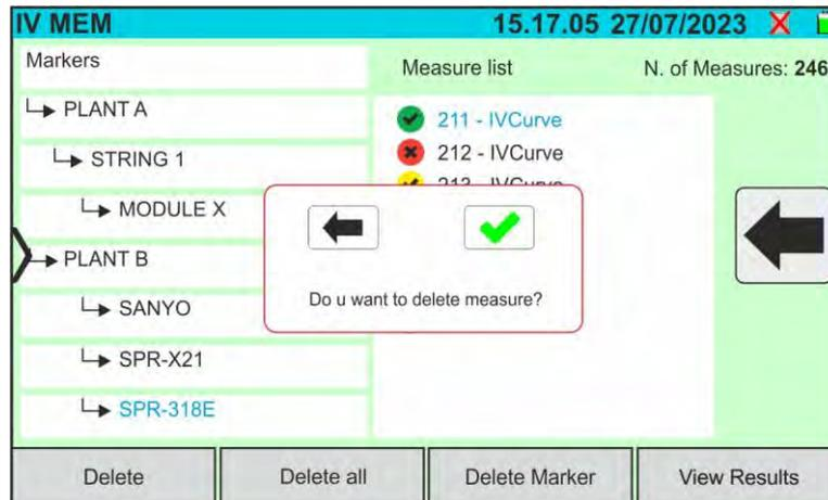
Fig. 79: Deleting a measurement result
