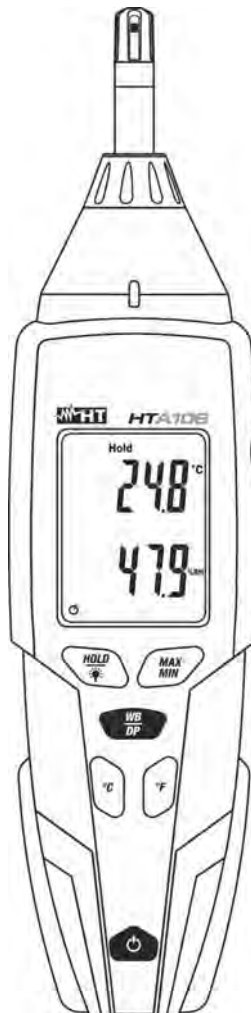
Fig. 3: Use of the instrument for air temperature/humidity measurement
