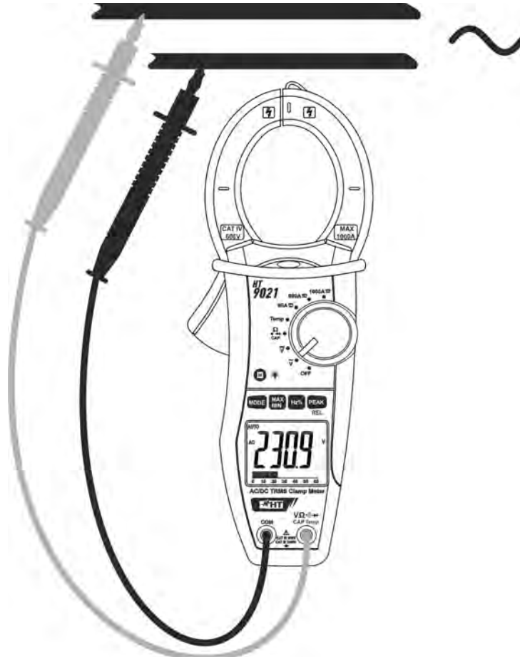
Fig. 3: Taking AC voltage measurements
