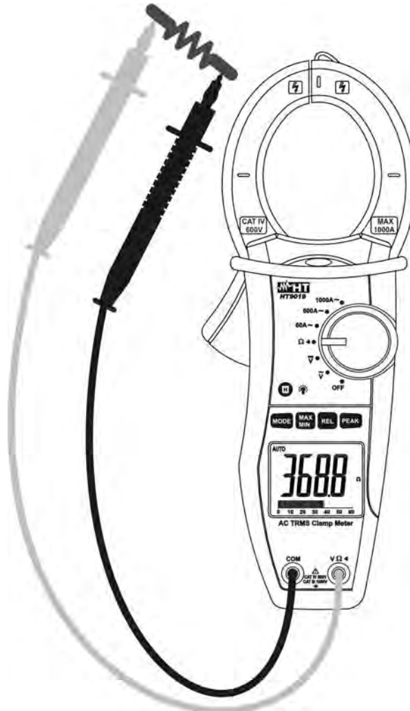
Fig. 5: Taking Resistance measurement and Continuity test
