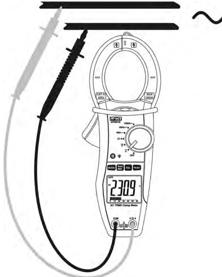
Fig. 3: Taking AC voltage measurements
