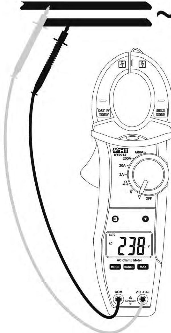
Fig. 4: Taking AC voltage measurement
