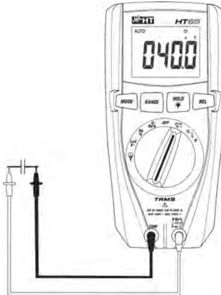
Fig. 8: Use of the instrument for Capacitance measurement
