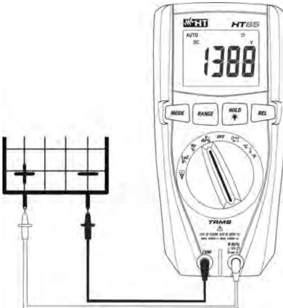
Fig. 2: Use of the instrument for DC Voltage measurement
