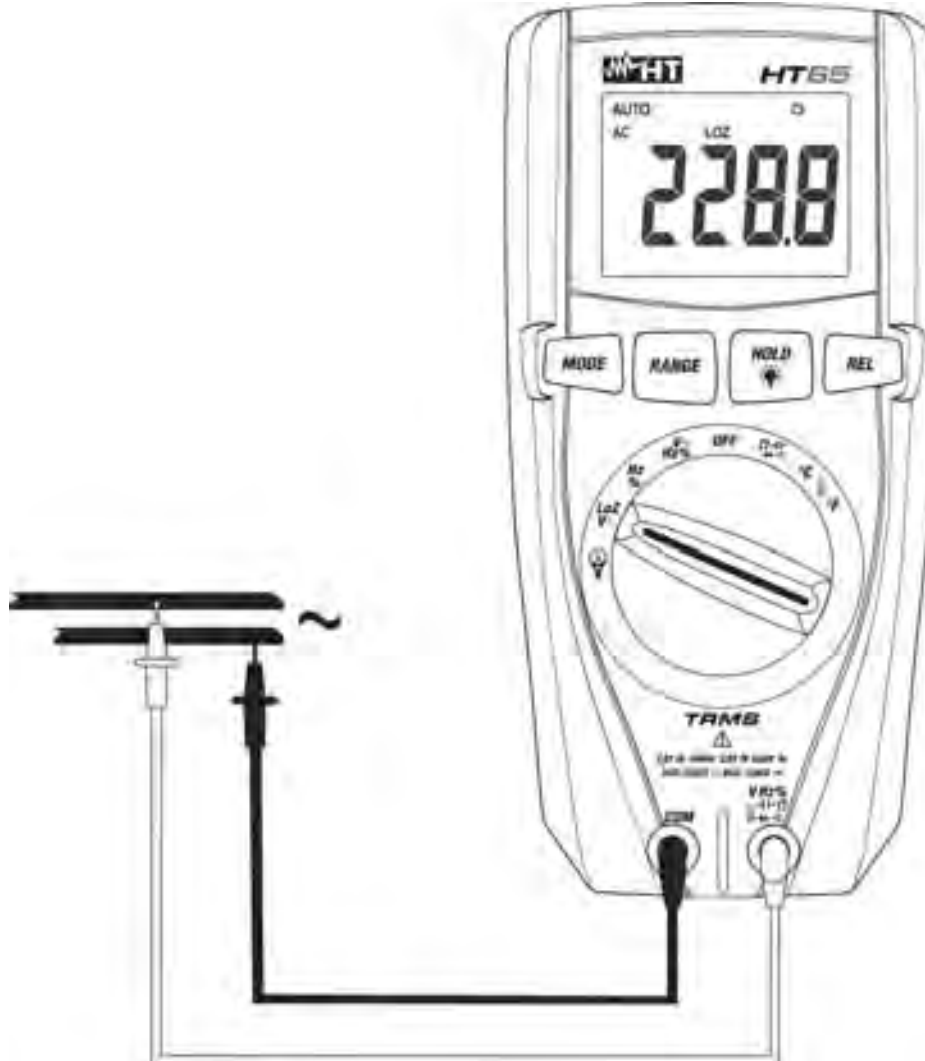
Fig. 4: Use of the instrument for AC/DC voltage measurement with low impedance (LoZ)
