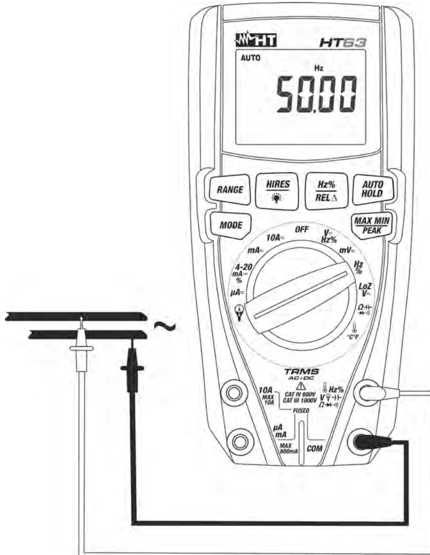
Fig. 5: Use of the instrument for frequency measurement and duty cycle test.
