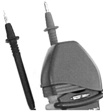
Fig. 3: Use of rubber test lead holster
