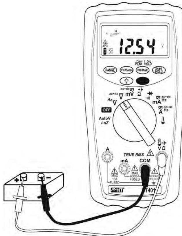
Fig. 2: DC voltage measurement
