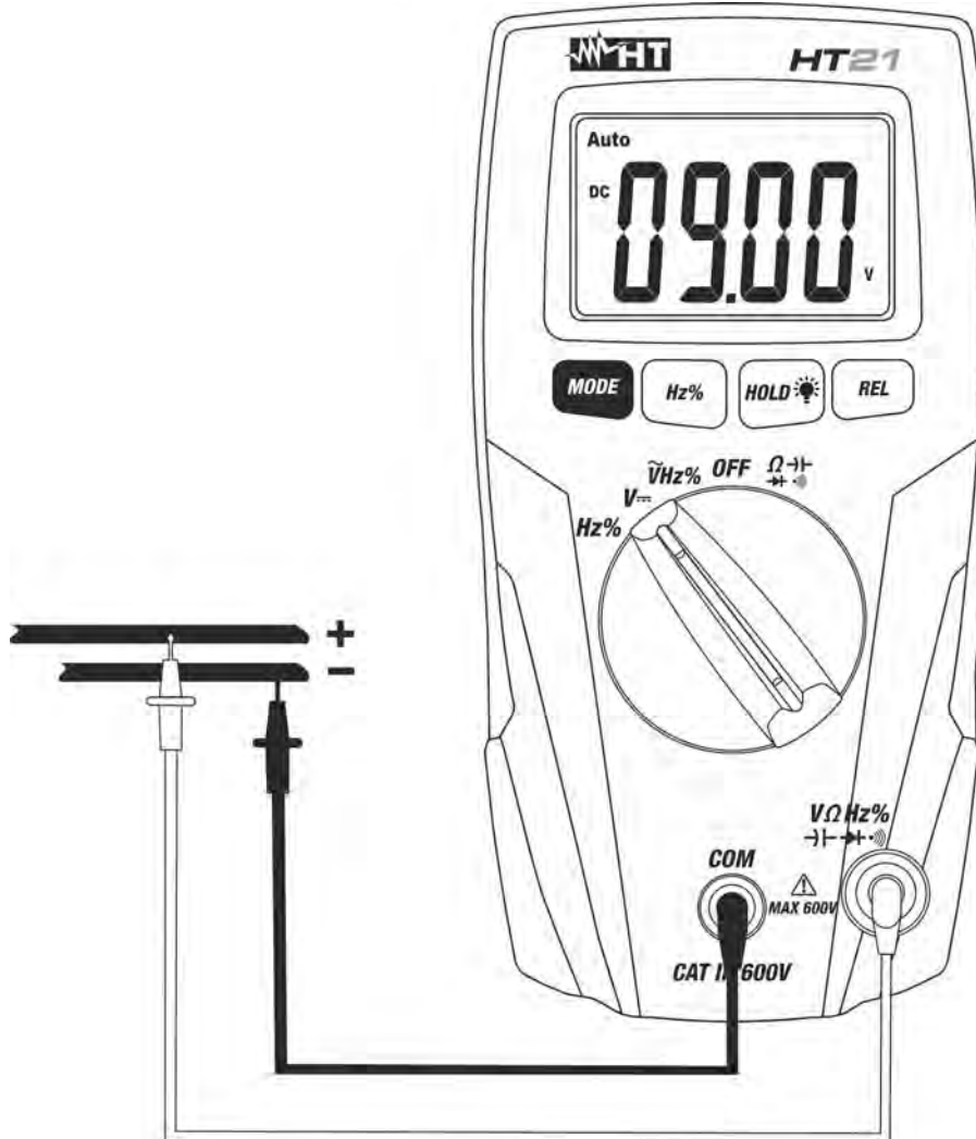
Fig. 2: Using the meter for DC Voltage measurement
