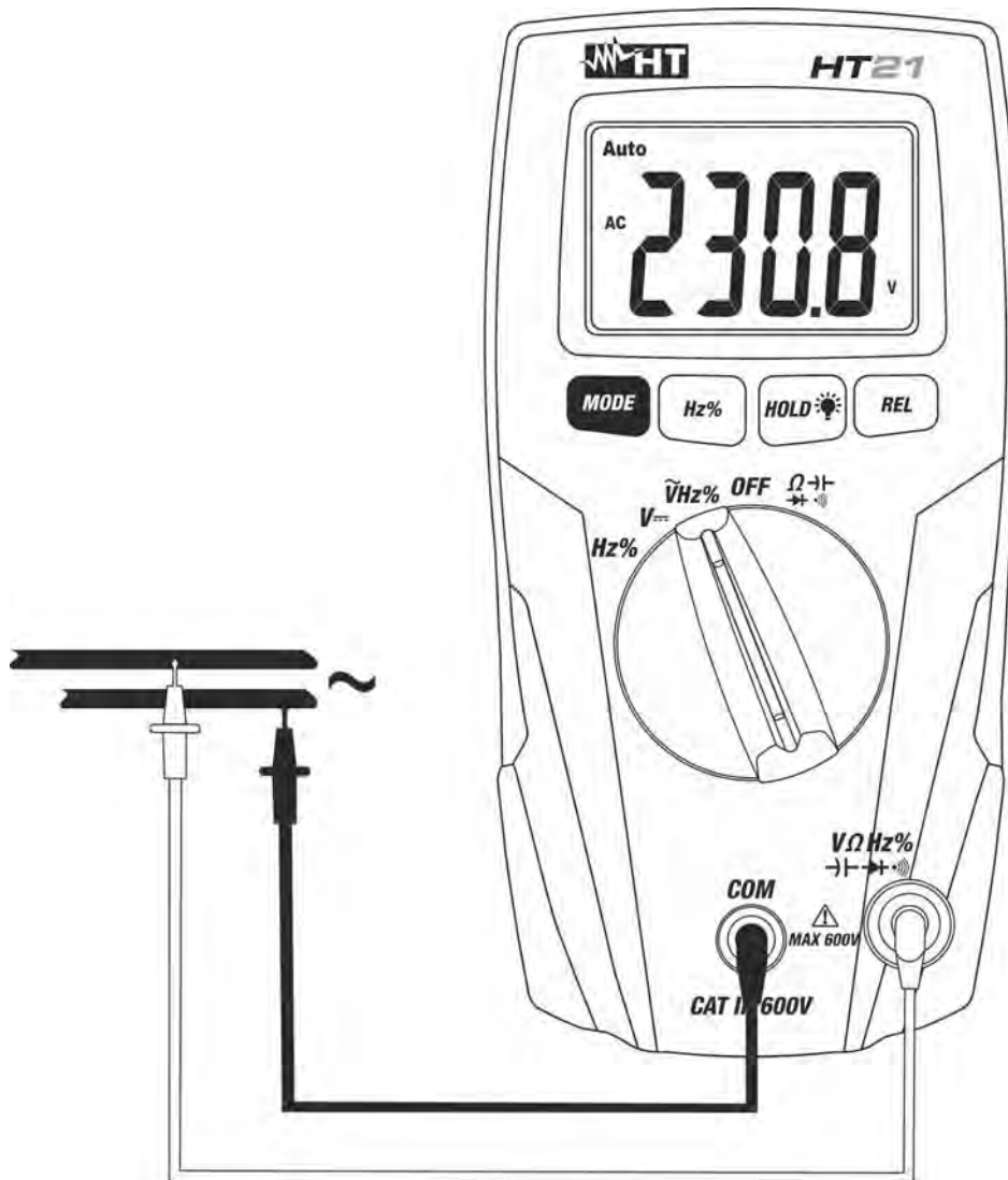
Fig. 3: Using the instrument for AC Voltage measurement
