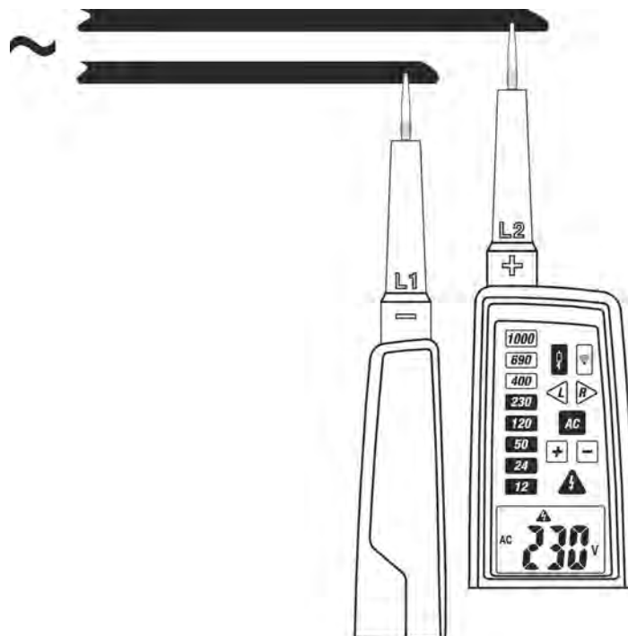
Fig. 6: AC Voltage measurement with low impedance value
