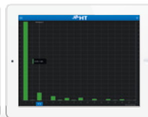
Current and voltage harmonics.
