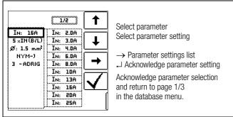
For example, nominal current values must be entered here for the selected electrical circuit. Measuring parameters which have been accepted and saved in this way are subsequently accepted by the current measuring menu automatically when the display is switched from the structure view to measurement.
