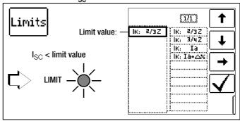
Short-circuit current  $I_{SC}$  is used to test shutdown by means of an overcurrent protective device. In order for an overcurrent protective device to be tripped on time, short-circuit current I<sub>SC</sub> must be greater than tripping current la (see table 6 in section 23.1). The variants which can be selected with the "Limits" key have the following meanings:
