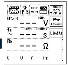
Amongst other values, touch voltage  $U_{I\Delta N}$  and calculated earthing resistance  $R_F$  appear at the display panel.
