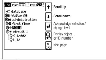
Use the  $\uparrow\downarrow$  keys in order to select structure elements. Change to the sub-level with the  $\downarrow$  key.
