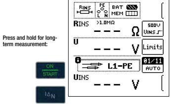
Quick polarity reversal if parameter is set to AUTO: 01/10 ... 10/10: L1-PE ... L1-L3
