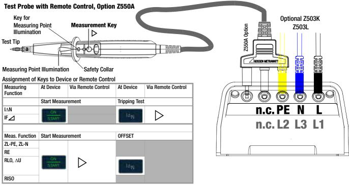
These connections are located under a protective rubber flap.
