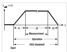
Suppression of RCCB tripping for RCCBs which are sensitive to pulsed current ot = 1
