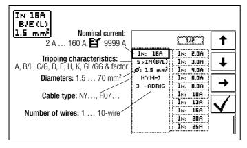
Press the softkey shown at the left in order to switch back and forth between the country-specific measuring adapter, e.g. PRO-Schuko measuring adapter (Z503K) / 3-pole measurement and the KS-PROFIT-
