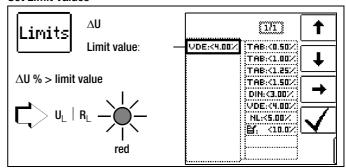
TAB Limit value per German technical connection conditions for connection to low-voltage mains between the distribution network and the measuring device
