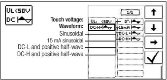
Sinusoidal (full-wave) Setting for circuit without RCD
