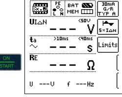
In both cases tripping time must be between 10 ms (minimum delay time for type G RCCBs!) and 40 ms.
