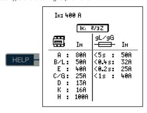
Key: Ia = breaking current,  $I_{SC}$  = short-circuit current,  $I_{N}$  = nominal current, tA = tripping time
