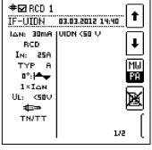
Scrolling amongst measurements is possible with the keys shown here:
