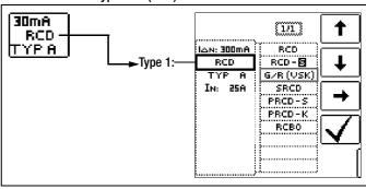
Touch voltage and time to trip can be measured in the G/R-RCD switch position.
