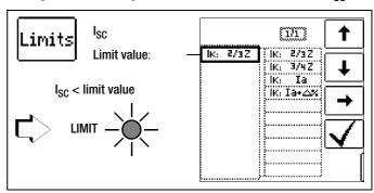
Short-circuit current  $I_{SC}$  is used to test shutdown by means of an overcurrent protective device. In order for an overcurrent protective device to be tripped on time, short-circuit current  $I_{SC}$  must be greater than tripping current Ia (see table 6 in section 23.1). The variants which can be selected with the "Limits" key have the following meanings:
