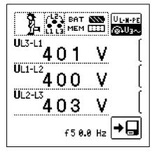
Clockwise phase sequence is required at all 3-phase electrical outlets.
