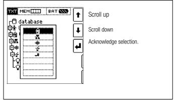
Select the desired object from the list with the ↑↓ keys and acknowledge with the
