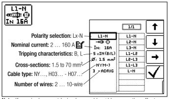
Note: If nominal current  $I_N$  is changed by  $\Delta U_{OFFSET}$ , the offset value is automatically adjusted.
