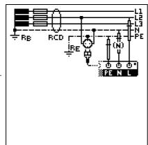
As a rule, the display for touch voltage is also 0.1 V, because the nominal residual current of 30 mA together with minimal loop resistance result in a very small voltage value:
