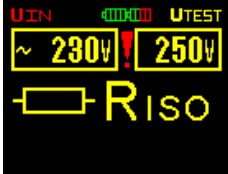
Fig. 4: (Interference) voltage display
