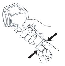
Before you discard the battery, apply insulation to the terminals with adhesive tape or equivalent materials.
