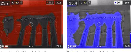
Above alarm: Highlights all pixels with a temperature above the specified temperature level.
