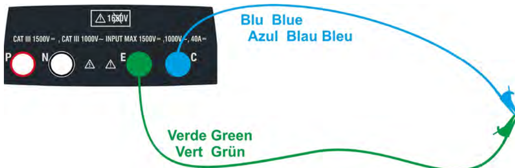
Fig. 5: Compensation of the measuring cables resistance
