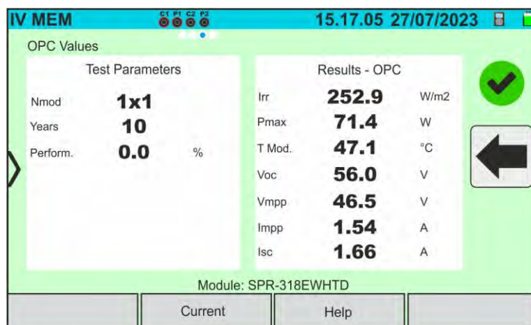
Fig. 75: Retrieving the I-V curve measurement results - Values @OTC
