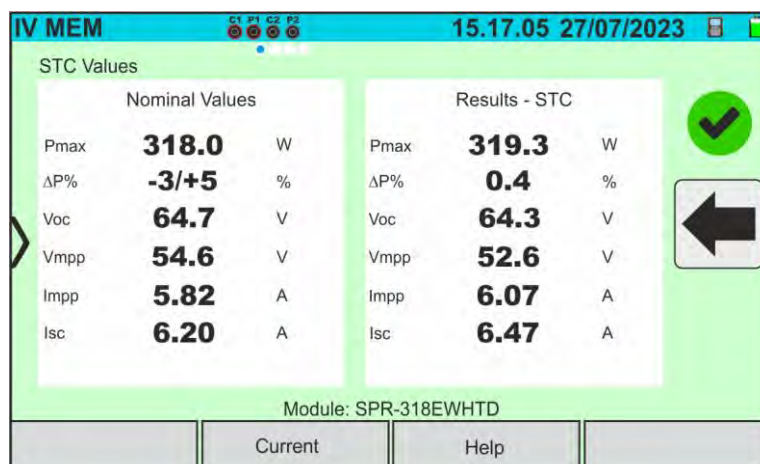
Fig. 72: Retrieving the I-V curve measurement results - Values @STC
