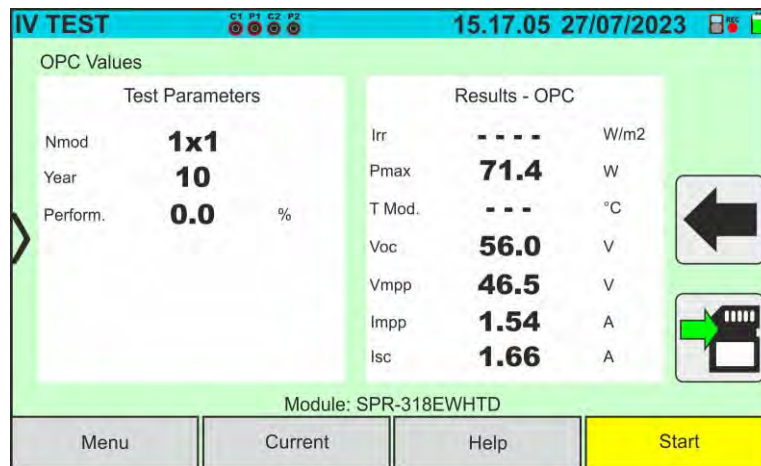
Fig. 43: I-V curve measurement result @OPC with synchronous recording
