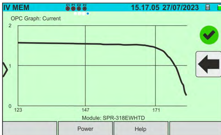
Fig. 76: Retrieving the I-V curve measurement results - Current curve @OPC
