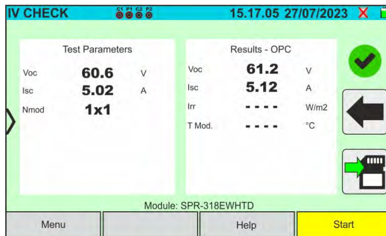
Fig. 50: Example of a positive IVCK test result - OPC values
