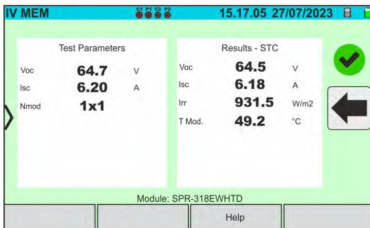
Fig. 78: Retrieving the IVCK test results @STC
