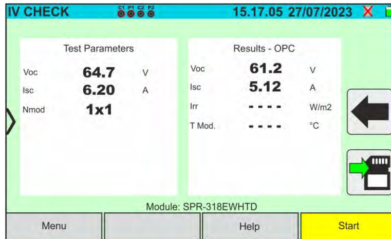
Fig. 60: IVCK test result @OPC with synchronous recording
