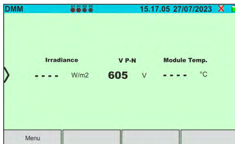
Fig. 14: DMM function measurement screen (SOLAR03 disconnected)
