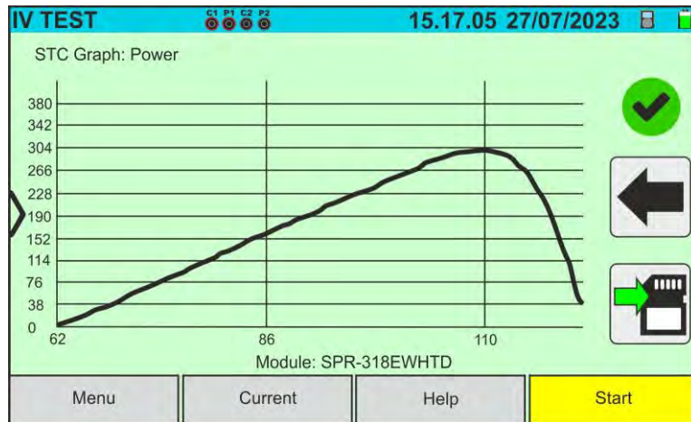
Fig. 40: Example of power measurement result - STC curve
