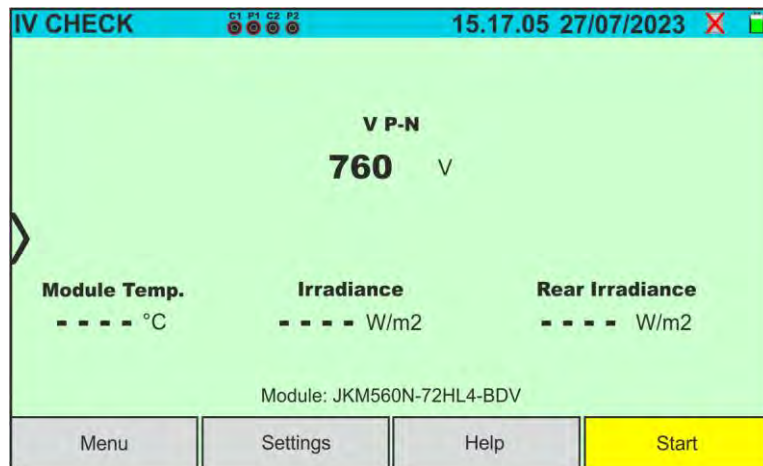
Fig. 47: Initial IVCK test screen without remote unit on Bifacial modules
