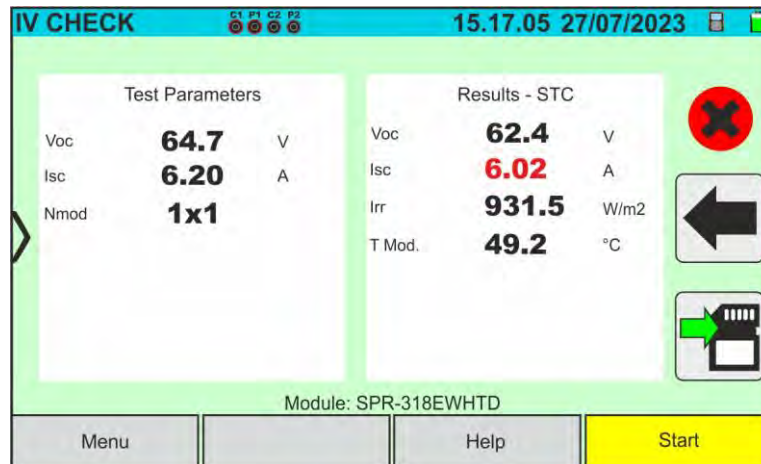
Fig. 59: Example of a negative IVCK test result - STC values
