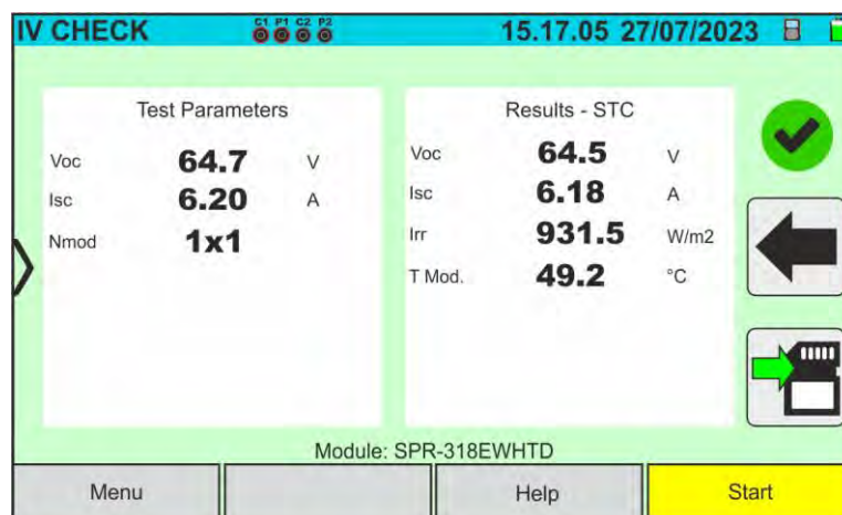
Fig. 58: Example of a positive IVCK test result - STC values
