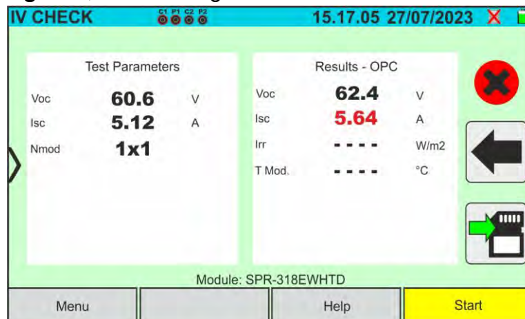
Fig. 51: Example of a negative IVCK test result - OPC values
