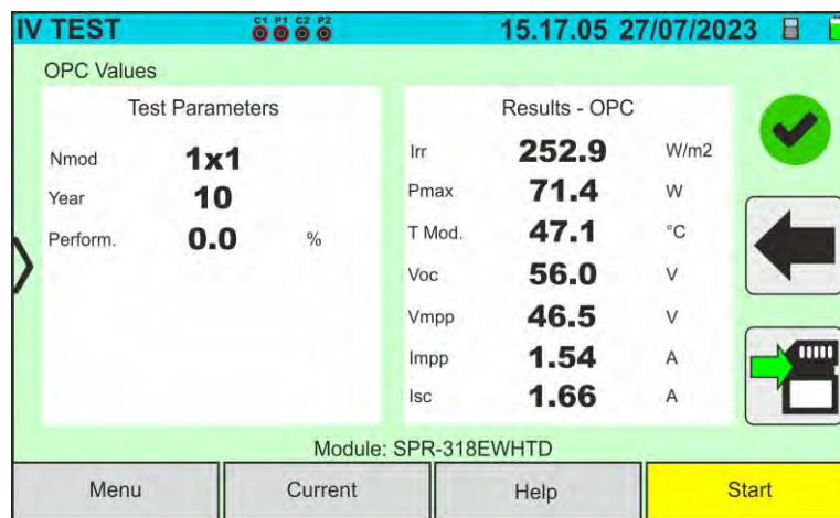
Fig. 38: Example of I-V curve measurement result - OPC values
