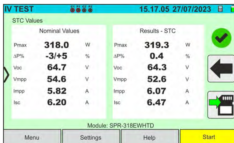
Fig. 37: Example of I-V curve measurement result - STC values
