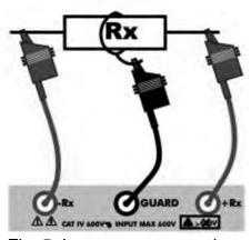
Fig. 5: Instrument connection
