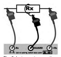
Fig. 6: Instrument connection
