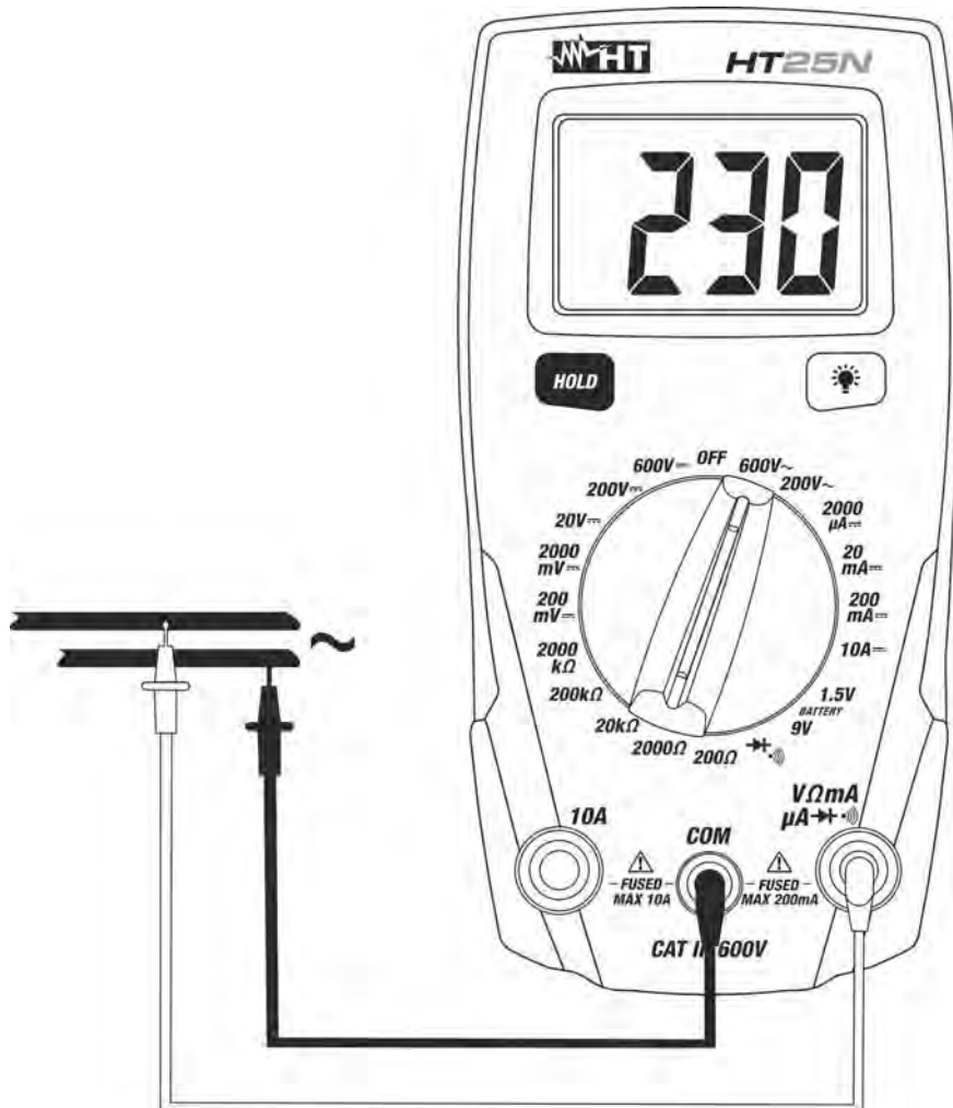
Fig. 3: Using the instrument for AC Voltage measurement
