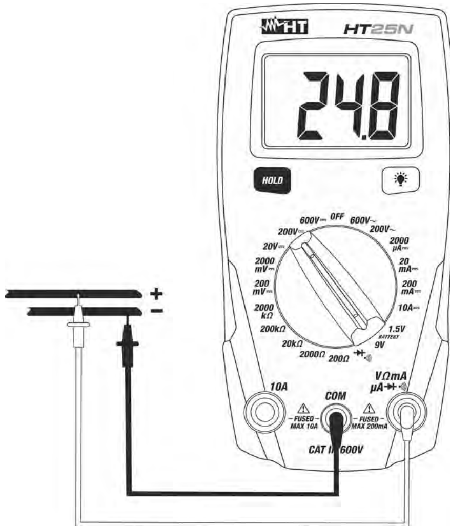
Fig. 2: Using the meter for DC Voltage measurement
