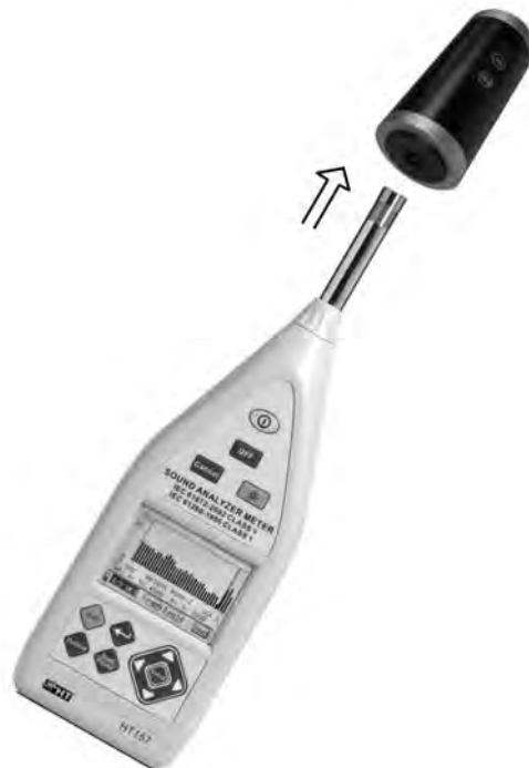
Fig. 36: Insertion of the calibrator HT151 into the instrument
