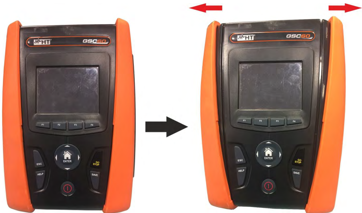
Fig. 45: Remove lateral half-shells
