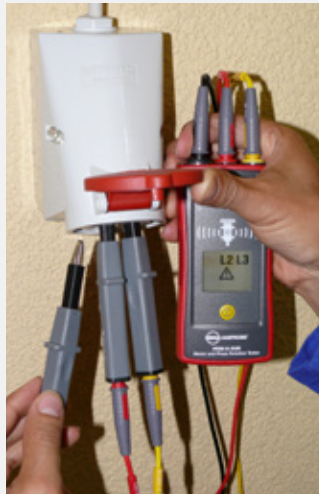
Validate receptacle wiring
