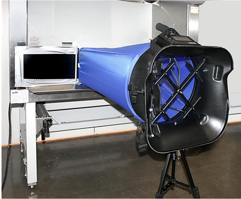
Figure 28: Adjust Height and Position of Telescopic Stand
