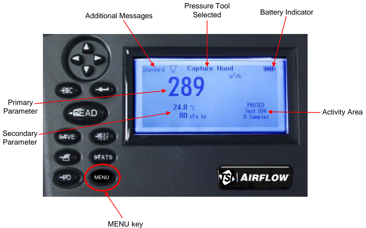
Figure 14: Keypad Functions
