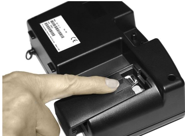
Figure 5: Battery Cover Removal
