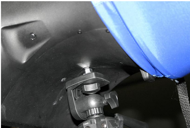
Figure 27: Mount Hood Base to Telescopic Stand
