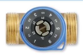
Handling has never been easier: The fitter can rapidly adjust the desired temperature of the mixed water in  $^{\circ}$ C by means of the dual scale; later on, only the adjusted scale value (1 – 6) is visible through the window in the cap.
