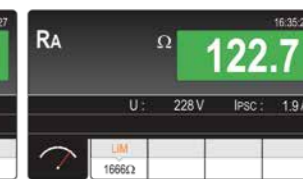
Measurement of overall earth resistance.
