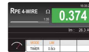
4-wire continuity test.
