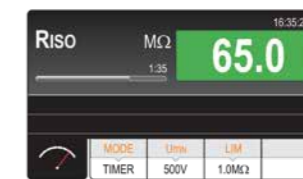
Measurement of insulation resistance.
