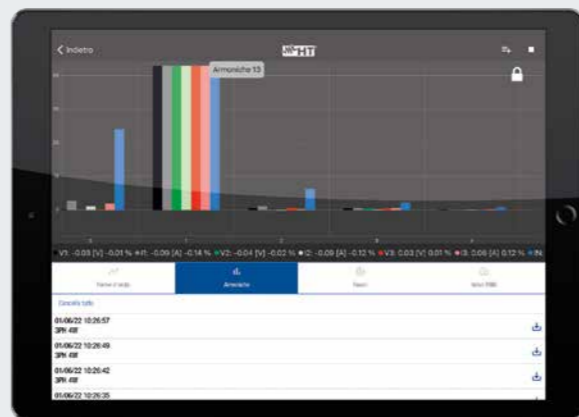
Current and voltage harmonics.
