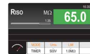
Measurement of insulation resistance.
