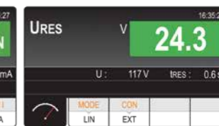
Residual voltage measurement.
