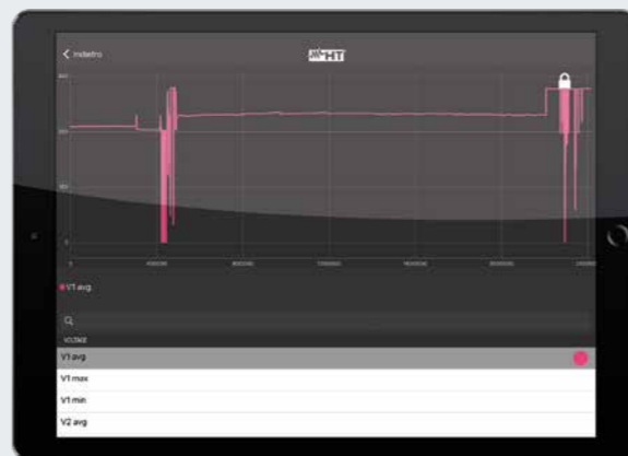
Zoom on a voltage and current drop.
