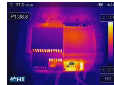
2 nd photo: thermogram of a power supply acquired with THT300.
