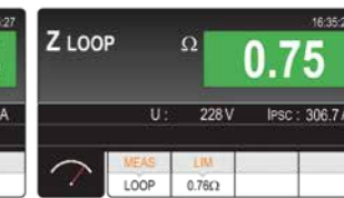
Measurement of Loop impedance.
