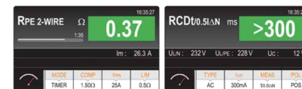
2-wire continuity test.
