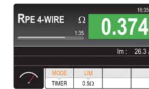
4-wire continuity test.
