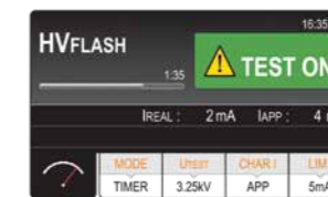
Dielectric strength test.
