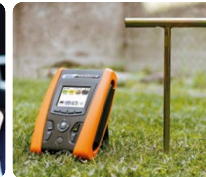
Measurement of earth impedance by voltammetric method.
