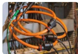
Flexible jaws for current measurement.
