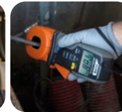
Earth resistance measurement with clamp T2100.
