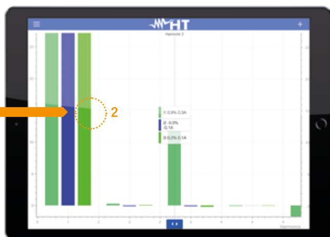
Jump function 2 It switches to harmonic values in real-time.
