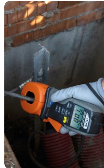
Measurement of earth resistance with Clamp T2100.
