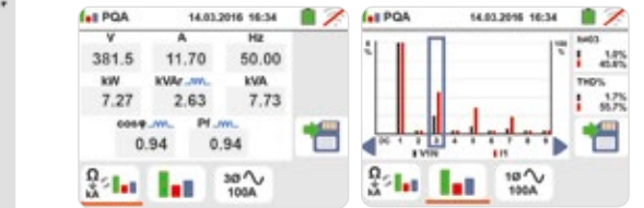
Power measurement. Power measurement: harmonics.
