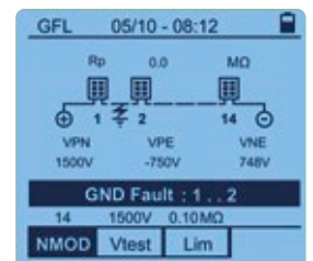
GFL (fault locator) function
