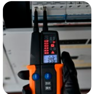
Measurement of phase sequence.
