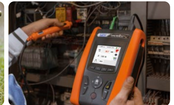
Start/stop measuring with remote lead PR400.
