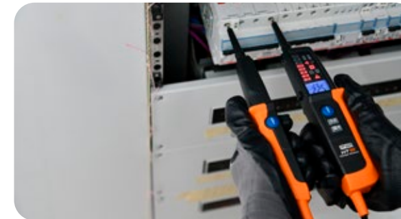
Phase detection function through conductive button.
