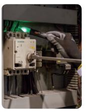
Step3 - If the green LED turns on with steady light, phase sequence is correct. If, however, the red LED flashes, phase sequence is incorrect.
