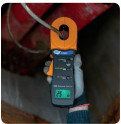
Measurement of earth resistance with Clamp T2100.
