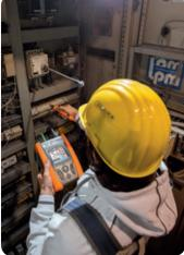
Start/stop measuring with remote lead PR400.
