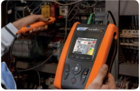
Start/stop measuring with remote lead PR400.
