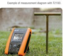
Measurement of earth impedance by voltammetric method.
